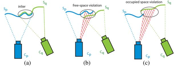
Figure 2. Geometric consistency: a) Consistent surfaces as  $S_p$  and  $S_q$  are close in  $C_p$ . b) Free space violation as  $S_q$  occludes  $S_p$  in  $C_p$ . c) Occupied space violation as  $S_q$  is not seen in  $C_p$ .
