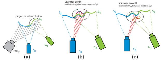
Figure 3. a) OSV due to projector occlusions are handled by projection. a) *type-I scanner error*:  $S_q$  occludes (incorrect)  $S_p$ , but phase is consistent in  $C_p$ . b) *type-II scanner error*: (incorrect)  $S_q$  occludes  $S_p$ , but phase is consistent in  $C_q$ .
