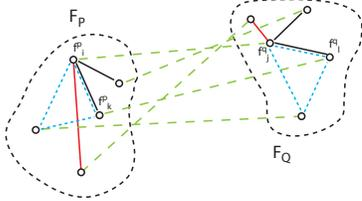
Figure 9. Correspondences of two features sets  $F_P$  and  $F_Q$  are shown in green. The *two* most distance-compatible correspondences of  $K_{ij} = (f_i^p, f_j^q)$  are shown in black, an incompatible correspondence red, and the most compatible triple in blue.
