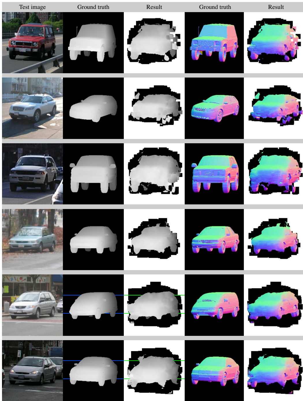
Fig. 7. Results for the car depth map and surface orientation experiments. From left to right: test image, ground-truth and output of our system for the depth map experiment, and ground-truth and output for the surface orientation experiment. The R, G, B colors represent the components of the surface normal according to Eq. 7. White areas are unlabeled and can be considered background.
