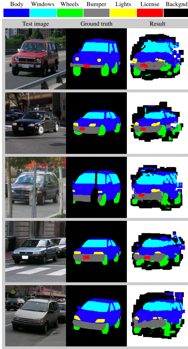
Fig. 12. Results for the car parts annotation experiment. From left to right: test image, ground-truth, and output of our system. White areas are unlabeled and can be considered background.
