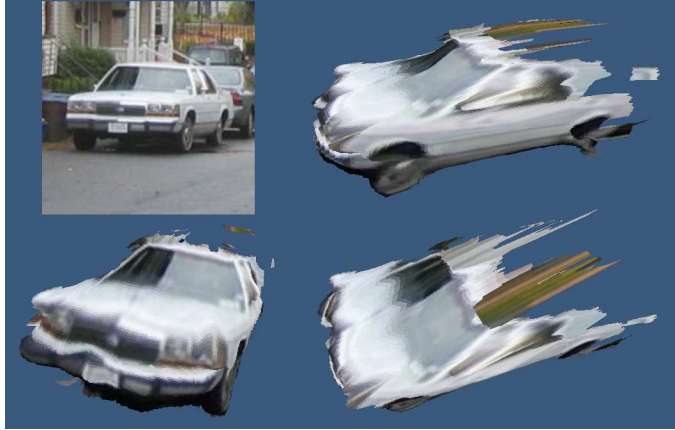
Fig. 10. Some views of a texture mapped 3D model, generated from the depth map of the recognized car in the top left corner.
