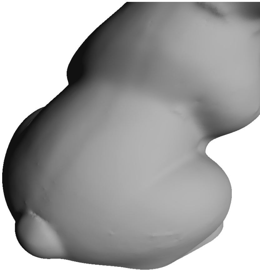
Figure 5.14: Closer look at the back of the bunny, where the vertical ridge due to manufacturing process is clearly visible.
