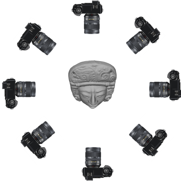
Figure 3.1: Visualization of a hypothetical setup: an object, surrounded by several cameras. Each camera provides normal estimates for the surface points, visible to the camera.
