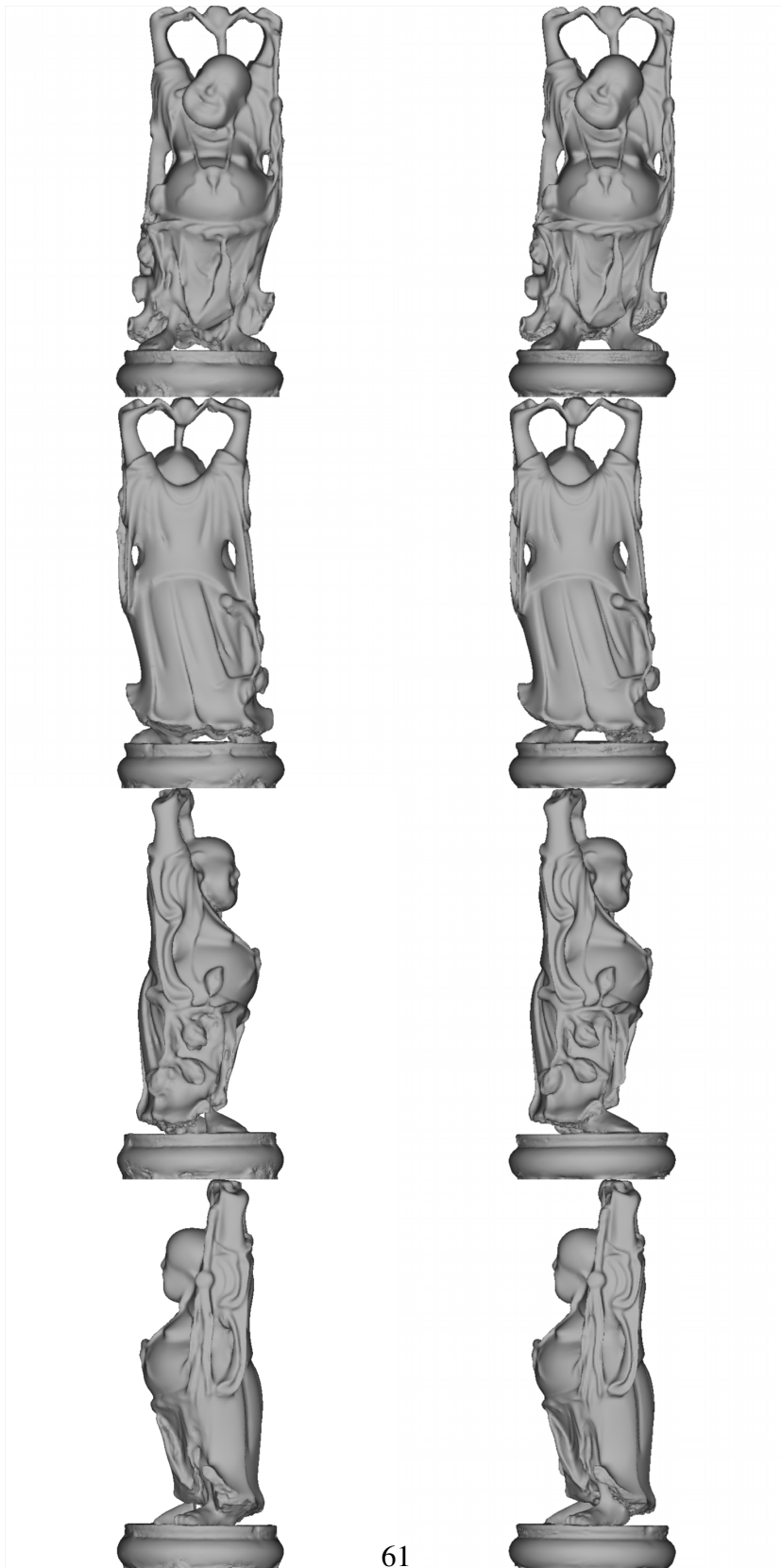
Figure 5.4: The Happy Buddha results: reconstructions using 10 cameras ( left column ) and reconstructions using 20 cameras ( right column ).
