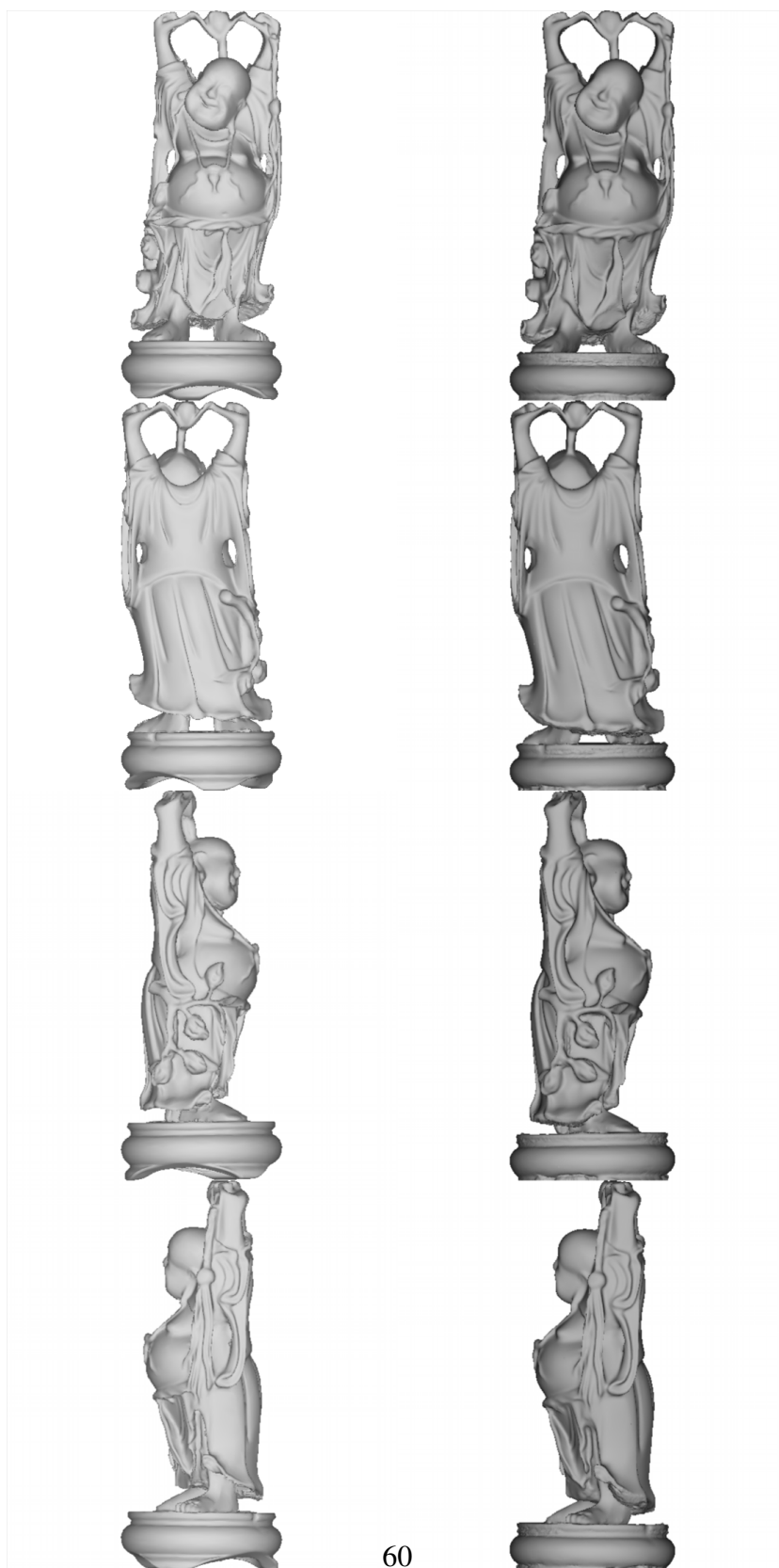
Figure 5.3: The Happy Buddha results: original model ( left column ) and reconstructions ( right column ), using 75 cameras.
