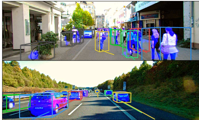
Fig. 1. We propose an approach to track generic objects in street scenes that goes beyond the capabilities of pre-trained object detectors. Our approach can handle a wide variety of static and moving objects of different sizes and robustly track them. Blue areas indicate potential object regions.
