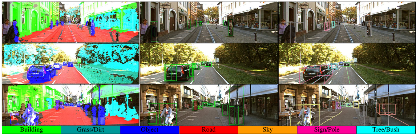
Fig. 6. Qualitative results on the KITTI tracking training set. Left: Semantic segmentation results. The label colors are shown in the color map at the bottom. Middle: Generic Object Proposals. Right: Tracking Results. The static objects are visualized with the gray bounding boxes.
