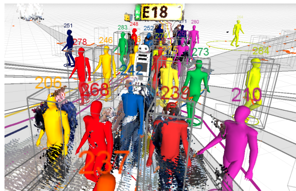
Fig. 1. Typical example of a crowded, dynamic situation in an airport terminal with frequent occlusions where we want to robustly and efficiently track persons from a first-person perspective with our mobile service robot platform, which can (barely) be seen in the center of the picture.
