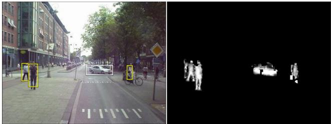
**Fig. 5.** Detections and corresponding top-down segmentations used to learn the object-specific color model.
