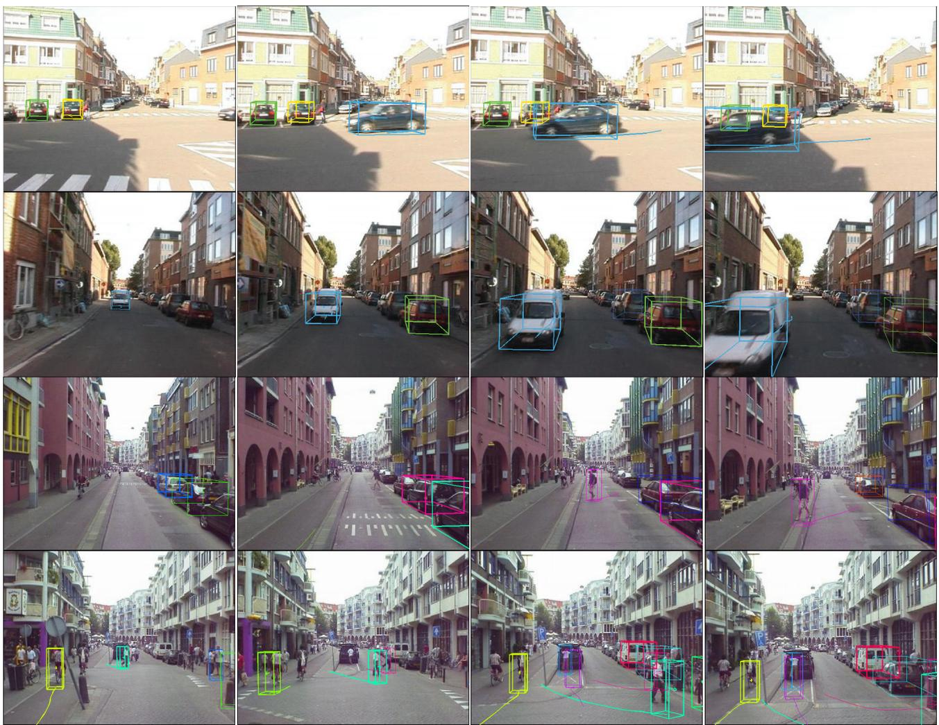
Fig. 16. 3D localization and tracking results of our system from inside a moving vehicle.
