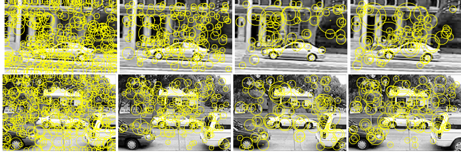
Fig. 1. Scale-invariant interest points found by (from left to right) the exact DoG, the fast DoG, the regular Harris-Laplace, and the fast Harris-Laplace detector on two example images (The smallest scales are omitted in order to reduce clutter).
