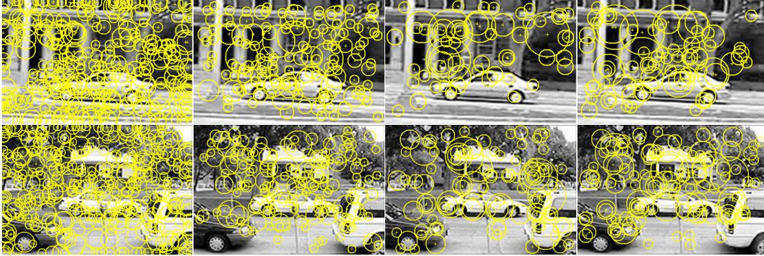
**Figure 7.1:** Scale-invariant interest points found by (from left to right) the exact DoG, the fast DoG, the regular Harris-Laplace, and the fast Harris-Laplace detector on two example images (The smallest scales are omitted in order to reduce clutter).
