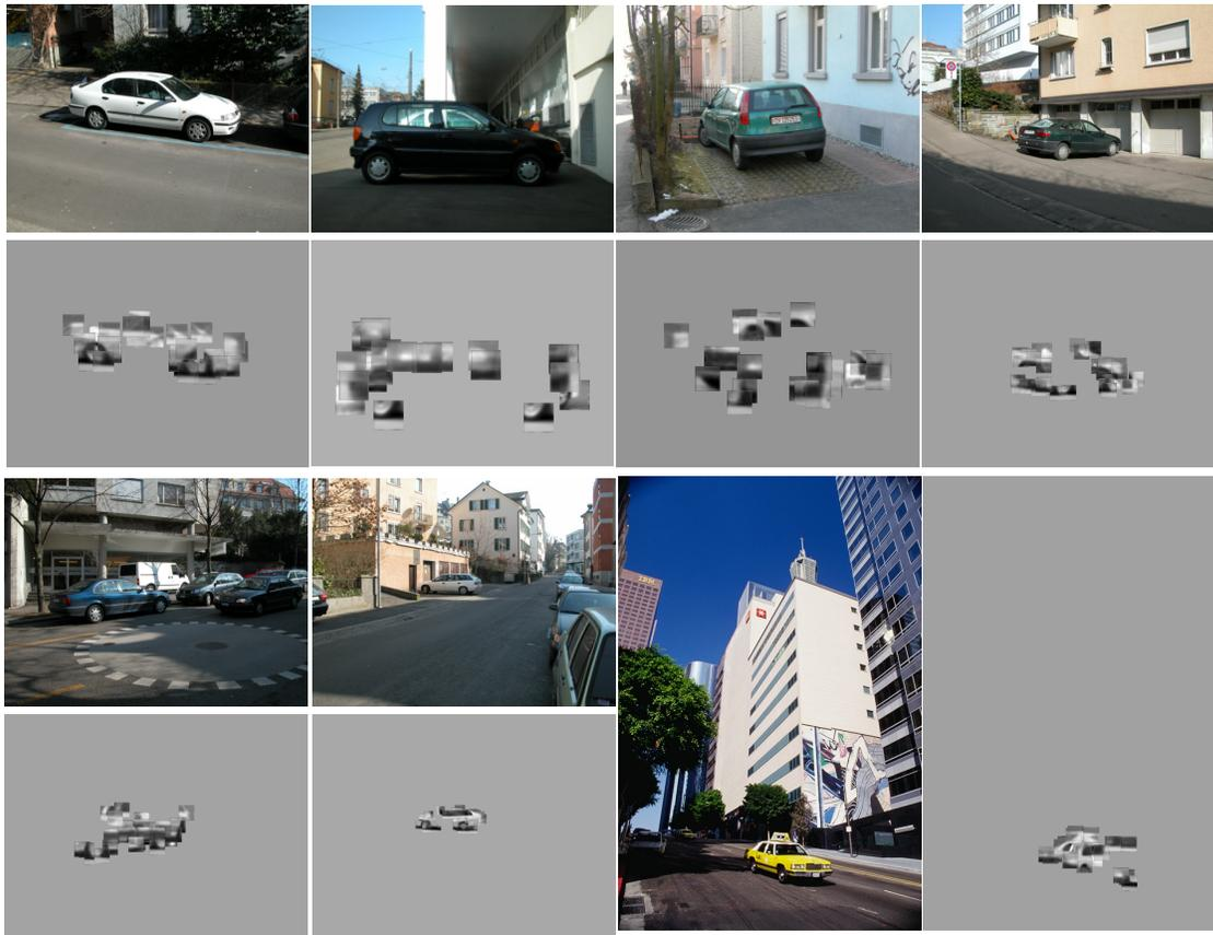
**Figure 5.4:** Some more examples of successful recognition results on real-world test images. The images show the support of the system's 1<sup>st</sup> hypothesis.
