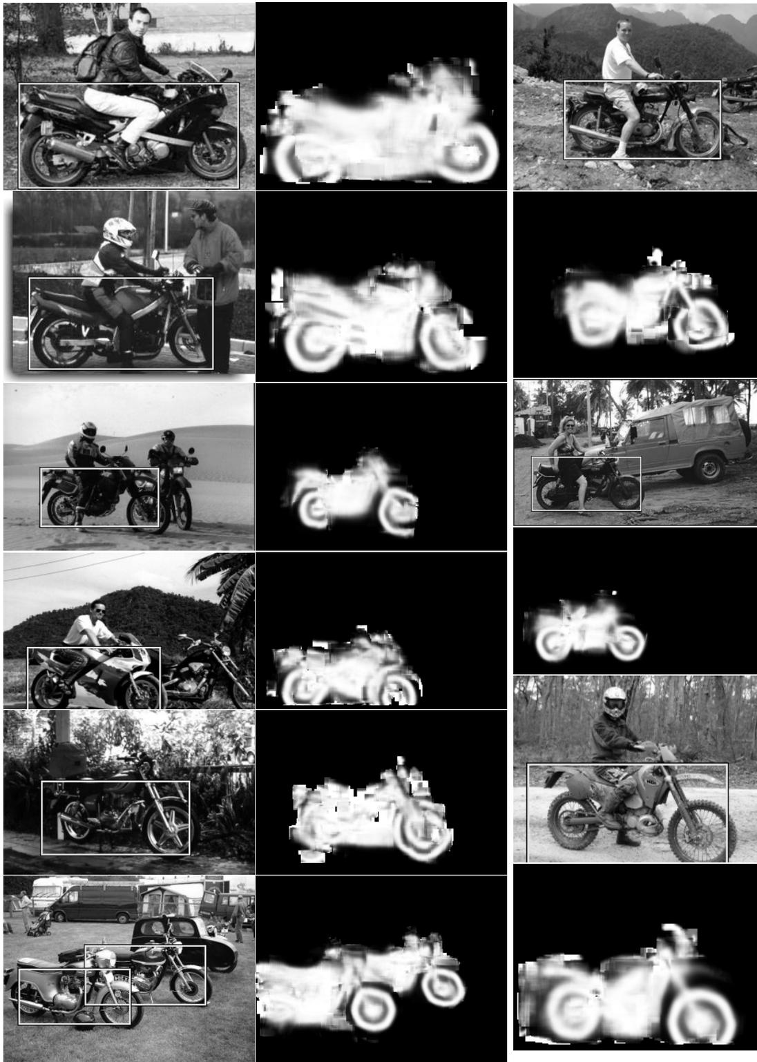
**Figure 8.15:** Example detection and segmentation results for motorbike images with partial occlusion and difficult backgrounds.
