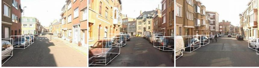
Fig. 7. Online 3D car location estimates (using only information from previous frames).
