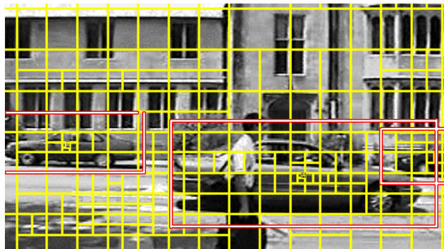
Figure 1. Adaptive subdivision of the search space. The object center serves as hypothesis parametrisation. Each yellow box corresponds to a set of hypotheses (which comprises objects whose center is within the box). The discretisation around object centers is much finer than on background regions.
