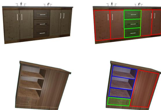
Figure 1: Semantic segmentation of modular furniture in RGBD images: Left column is the input front face of the furniture and right column is the segmentation output (door, drawer and shelf).
