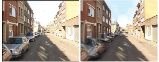
Figure 4. Left: An image taken from the original survey video. Right: A rendered image taken from the reconstructed 3D model from the same camera position.
