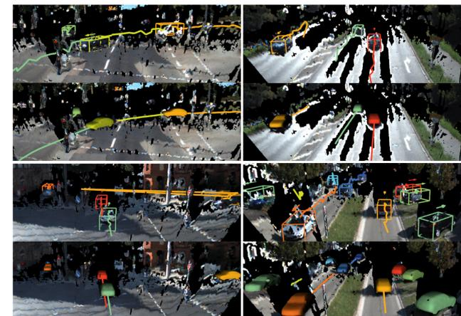
Qualitative Results. Top row: Input consisting of stereo reconstruction and tracked detections. Bottom row: Full shape reconstruction and improved pose estimations.
