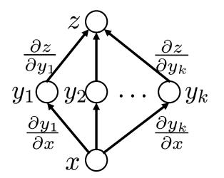
$$\frac{\partial z}{\partial x} = \frac{\partial z}{\partial y_1} \frac{\partial y_1}{\partial x} + \frac{\partial z}{\partial y_2} \frac{\partial y_2}{\partial x} + \dots$$
