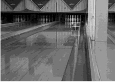
Crosshair indicates results of Hough transform, bounding box found via motion differencing.
