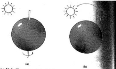
**Figure 12-2.** The optical flow is not always equal to the motion field. In (a) a smooth sphere is rotating under constant illumination—the image does not change, yet the motion field is nonzero. In (b) a fixed sphere is illuminated by a moving source—the shading in the image changes, yet the motion field is zero.
